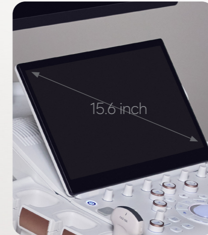
15.6" tilting touchscreen for optimal viewing
